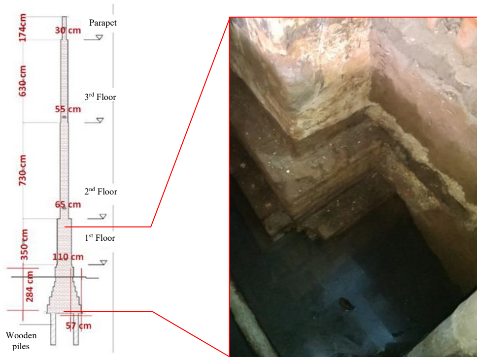
Fig. 7. Masonry Wall Section (Left) and Brick Foundation, Construction Technology of the Past (Right) Source: Kementerian Keuangan (2020) (Left) and Author(s) (2020) (Right)
