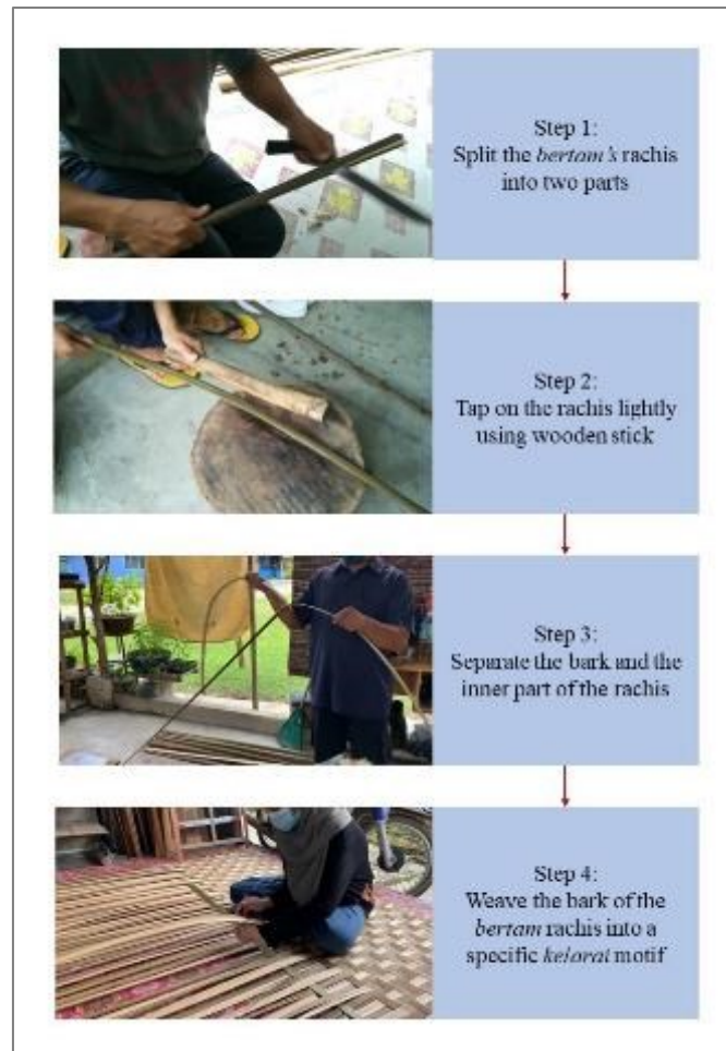
Fig. 4. Making Process of Kelarai Bertam Wall
